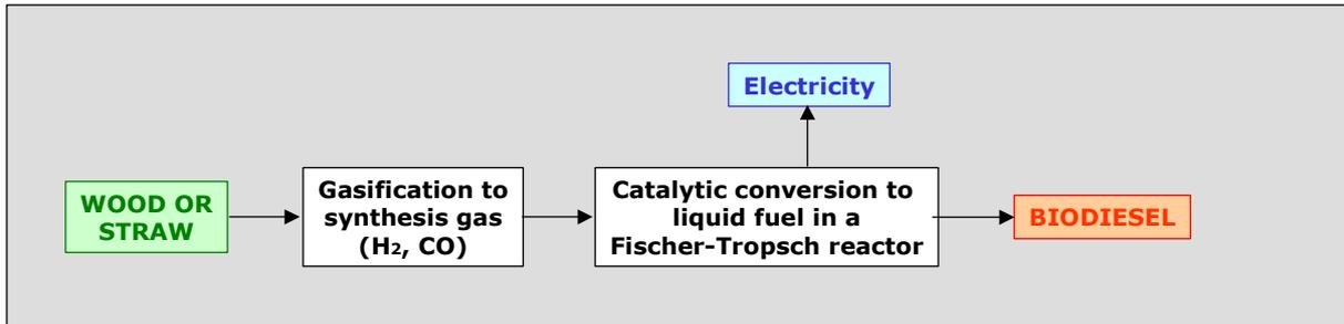
**Figure 2.6: Production of biodiesel by gasification and Fischer-Tropsch**
