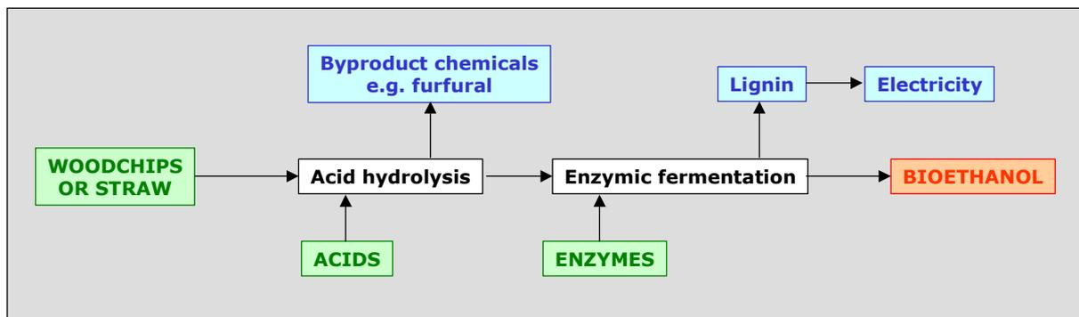
**Figure 2.2: Production of bioethanol from wood or straw by acid hydrolysis and fermentation**
